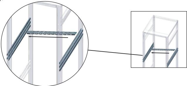
2) Fully insert into the opposite side rackrail slots, and then push into place to lock the accessory. The Lever Lock™ will 'click' into place when engaged.
