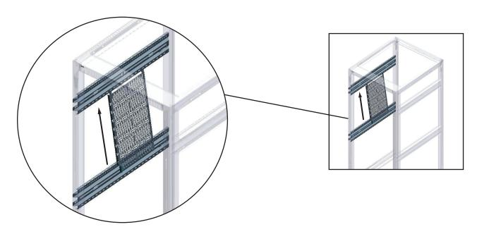
2) Fully insert into the top rackrail slots, and then push down into the corresponding slots in the lower rackrail bracket to lock the accessory into place. The Lever Lock™ will click into place when engaged.
